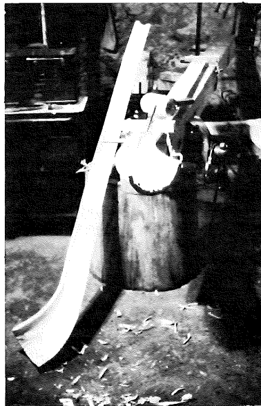
The lower section of the second horn nearing completion. The piece being worked is lashed to a heavy timber for stable positioning.
