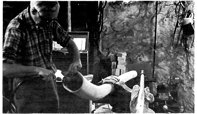
Dressing the bell with a rotary drum sander.
