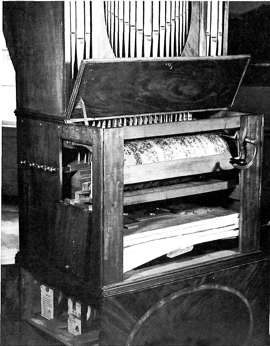
Courtesy of New York State Historical Association The pinned cylinder of the Howe barrel organ in Cooperstown.
