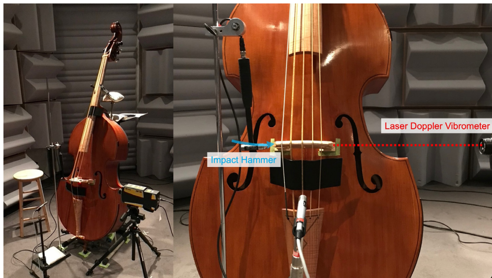
Figure 2. Setup for bridge admittance measurements (left), and close-up showing impact hammer and LDV alignment with the bridge (right).
