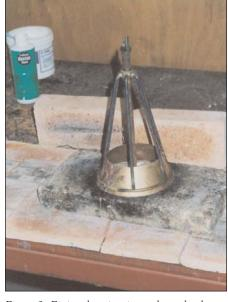
Figure 3. Fitting the wire rim to the garland.
