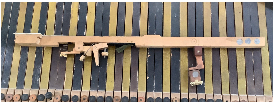
Figure 10. Spring-returned levers and damper assembly mounted beneath a lead-weighted key. Yellow and black paper strips distinguish natural and accidental keys, held down by leather nuts on their balance pins.
