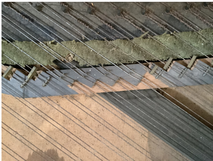
Figure 6. Pairs of bridge pins over a section of the bridge notched to accommodate an iron strut, flanked by sections with T-shaped brass pins pressing bichords onto bent, flattened nails. Observe the angled joint (left) in the bridge, and hitchpins embedded in the bentside frame rail.
