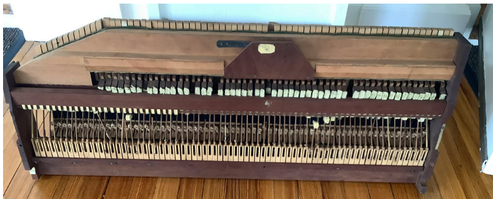
Figure 11. Bottom of the action frame. The white rectangles are dampers. Below, the hammers pivot in forked flanges. The trapezoidal, pedal-operated batten lowers the leather-hinged mute rail and is returned by a leaf spring.
